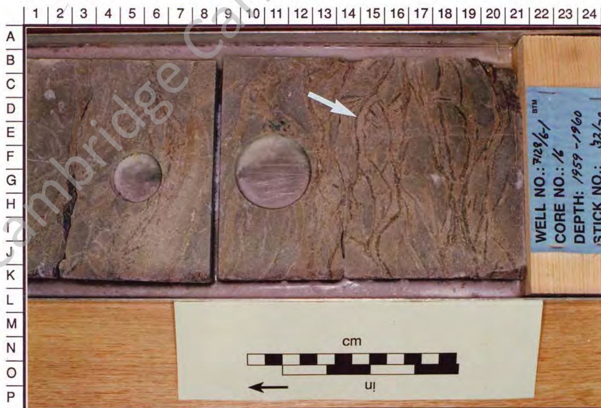
Plate 2: Core 16, Sakmarian to Asselian, 1959.9m. M-boundstone with large Palaeoaplysina plates (E14) and micrite (grey). Remainder of boundstone is mainly internal sediment. (See also Figure 13).
